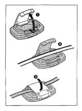
Attaching to the Strap Open the buckle ①, insert the strap ②, and close the buckle ③. The remote control can be attached to round straps with a diameter of 3 ~ 5 mm (0.12 ~ 0.2 in) and flat straps with a thickness of 1.2 ~ 2 mm (0.05 ~ 0.08 in) and a width of 6 ~ 12.5 mm (0.24 ~ 0.5 in).
